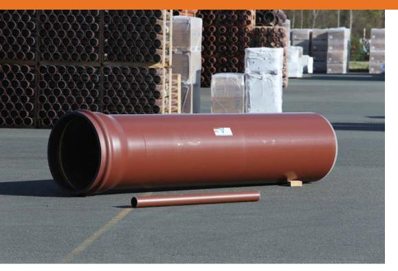
The Funke HS pipe range is a comprehensive sewer pipe system with outstanding performance. Pipes are available in diameters from 110mm to 800mm and SN12 & SN16 ratings, complemented by a comprehensive range of SDR34 fittings including bends, junctions and chambers, and innovative pipe connections which enable the system to integrate with existing pipe networks of various materials.
